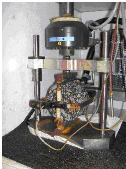
Figure 2: Indirect Tensile Tests
