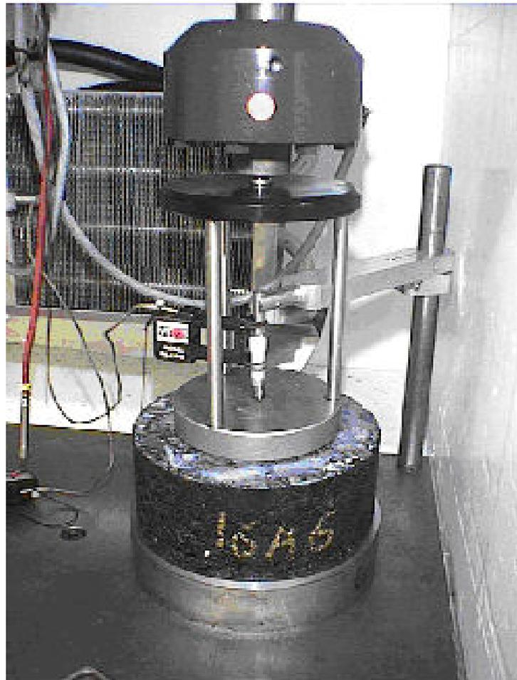
Figure 3: Creep test
